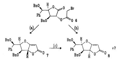
(a) PPh<sub>3</sub>, CH<sub>3</sub>CN, then DBU, reflux, 30 min (88%), (b) PPh<sub>3</sub>, CH<sub>3</sub>CN, then excess DBU, reflux, 30 min (81% combined), (c) catalytic DBU, CH<sub>3</sub>CN, reflux.
